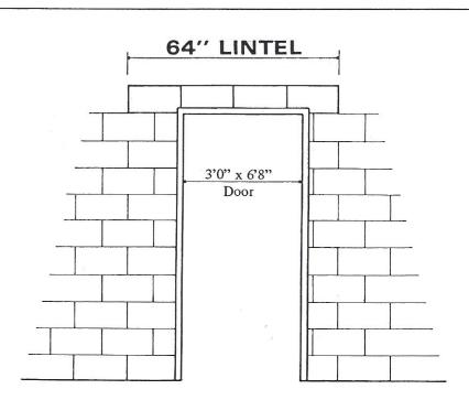
Lintels 64" long will course to most masonry openings up to 3'4" wide, Contractor and supplier to work together to insure proper coursing. Shop drawing to be provided by request.
