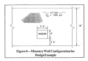
$D_{wall} = 58.2 \text{ lb/ft}^2 (3 \text{ ft}) = 175 \text{ lb/ft} (2.5 \text{ kN/m})$
