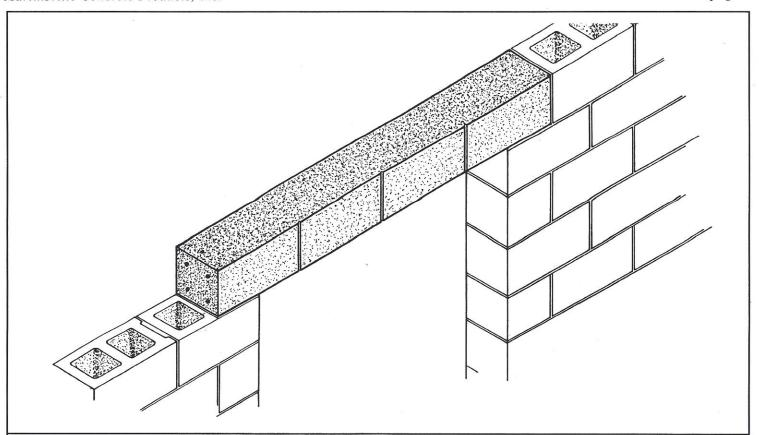
Lintels are professionally designed, laboratory tested and textured to match lightweight and heavyweight concrete block. Each unit can be marked for identification to insure proper handling and use. Special sizes or aggregates will be made on submission of a detailed specification. IMPORTANT – never store, handle, or use lintels flat and always install them within the limits of safe load tables for proper appliable loads and weights per foot.
