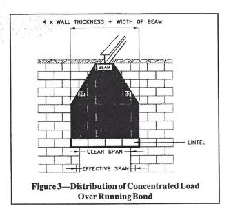
Concentrated loads are assumed to be distributed downwards at an angle of thirty degrees from the vertical on each side of bearing, with maximum length equal to four times the wall thickness plus the width of the bearing, as shown in Figure 3. This is then resolved onto the lintel as a uniform load. The magnitude of the load per unit length is determined by dividing the
